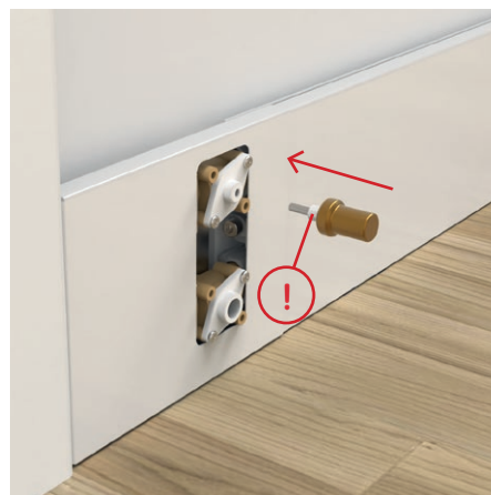
Insert the wax element into the TRV valve before fitting the TRV knob. Do not forget the white spacer!
